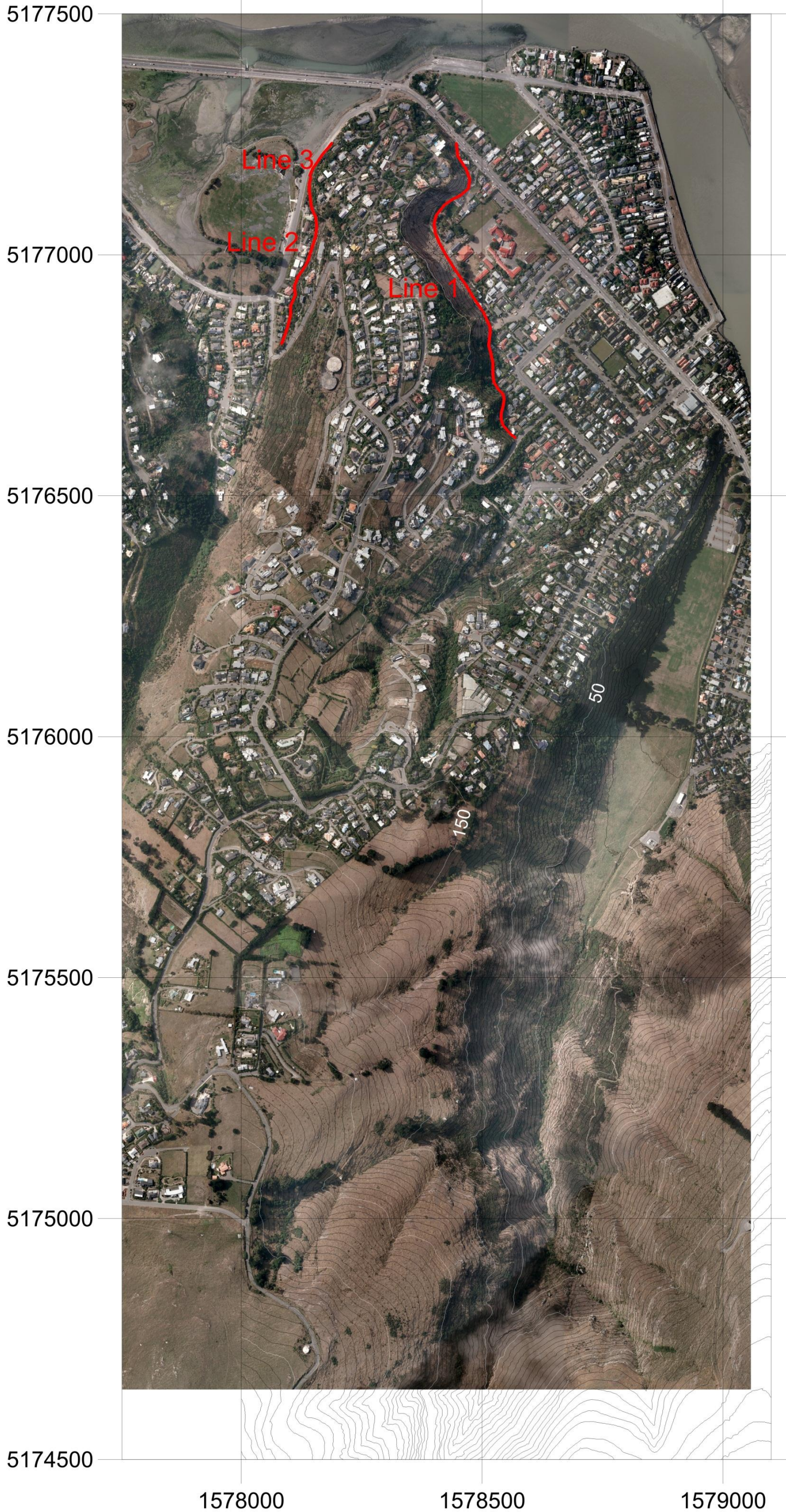
Figure 2 - Recommended Location of Rockfall Barriers
