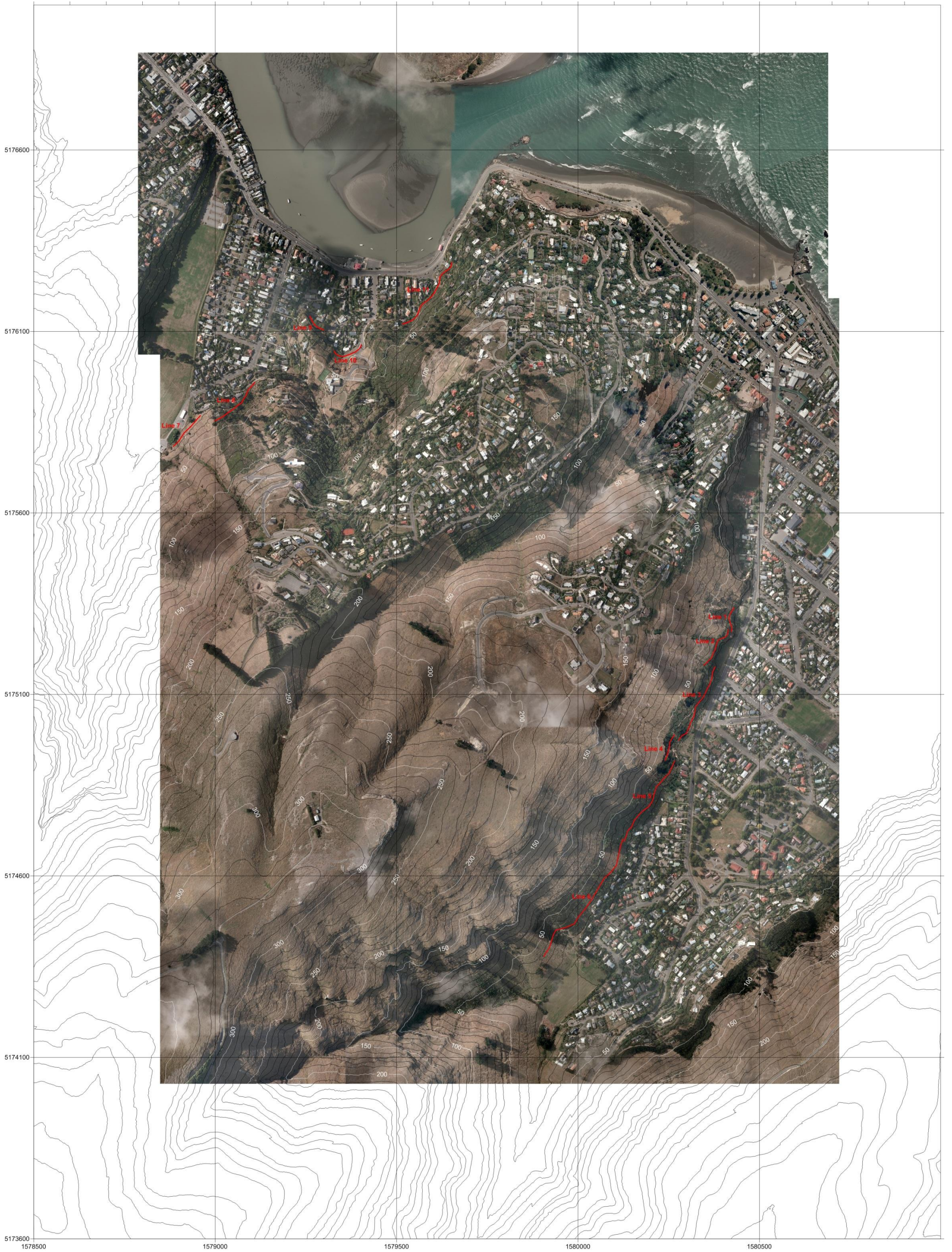
Figure 2 - Recommended Location of Rockfall Barriers
