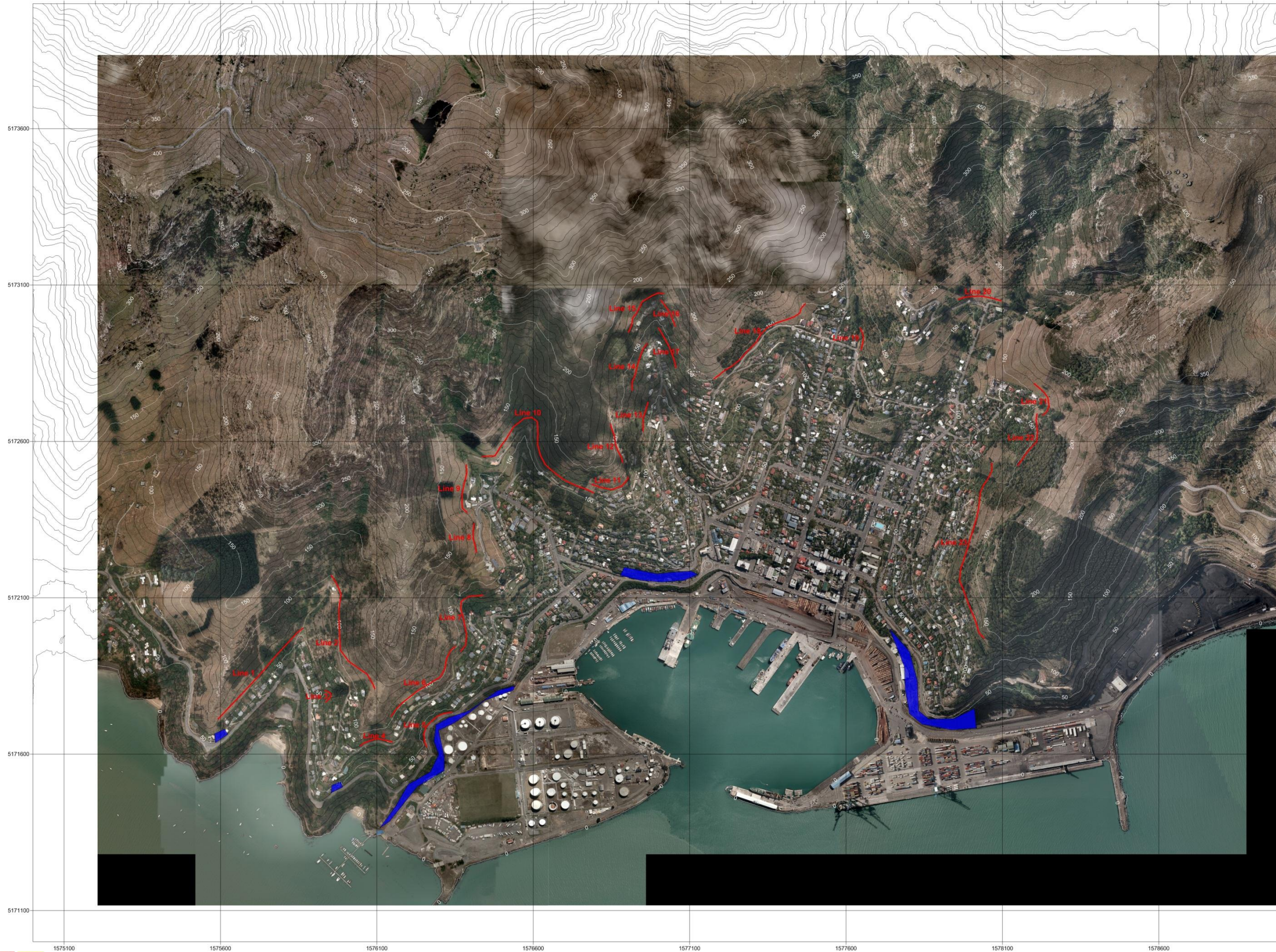
Figure 2 - Recommended Location of Rockfall Barriers
