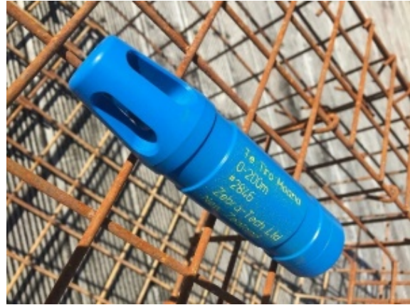
Figure 98: A temperature sensor used in the Moana Project. Image credit: 2018 MetOcean Solutions/ Meteorological Service of New Zealand (CC BY-NC-SA 4.0).
