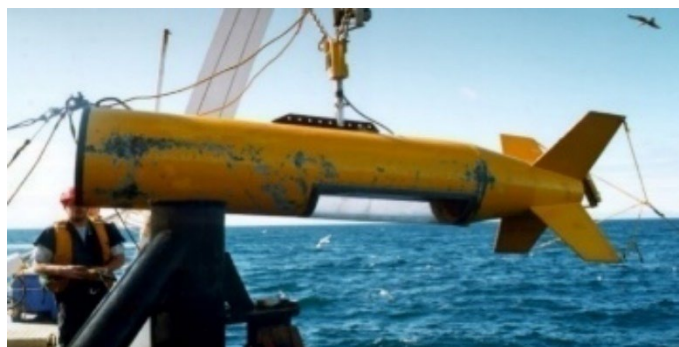
Figure 102: Deep tow body being deployed.
