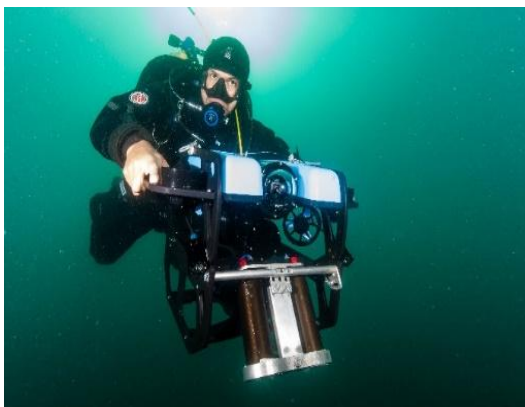
Figure 115: Underwater stereo-camera used for image capture fieldwork. The camera was operated by NIWA scientific divers, ‘flying’ the camera along pre-deployed transect lines at each site, with the camera set at forward looking and vertical face-down angles. Image credit: James Williams.
