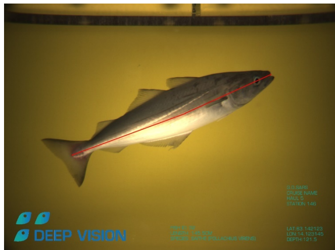
Figure 125: A fish with length measurement captured by the Deep Vision system. Image credit: Deep Vision.
