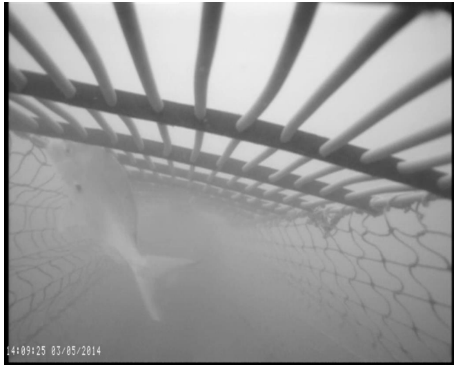
Figure 111: Underwater screen shot of a snapper attempting to escape in a trawl fitted with a novel escape panel. Image credit: NIWA.
