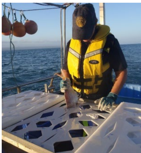
Figure 112: Collecting "artificial" selectivity data from "fall-through" experiments. Photo credit: Jure Brčić /NIWA.
