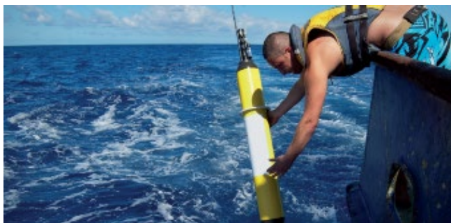
Figure 95: Deploying an Argo float, part of a worldwide network of ocean sensors collecting data. Image credit: NIWA.
