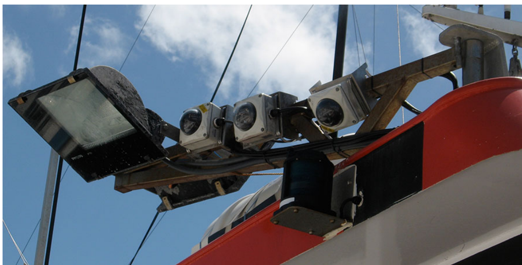
Figure 127: Electronic monitoring cameras onboard a fishing vessel. Image credit: AFMA.
