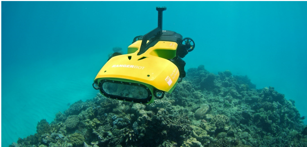
Figure 149: The autonomous RangerBot that can identify invasive crown-of-thorns starfish on the Great Barrier Reef. Image credit: Queensland University of Technology.
