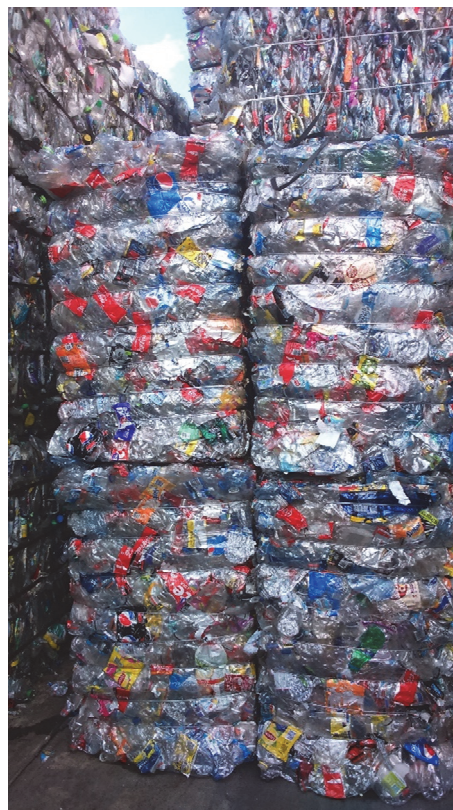
Figure 13 Bales of clear PET (# 1) ready to be sent for recycling. Photo credit: Stephen Harris
